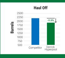
With less fluid being removed, there was an 11.9% reduction in barrels hauled off, contributing to operational savings and a greener footprint at the Anadarko-Woodford Basin site. With an average cost savings of \$27,000 per well, Derrick's Hyperpool came out on top when put side-by-side with the competitor's latest shaker.
