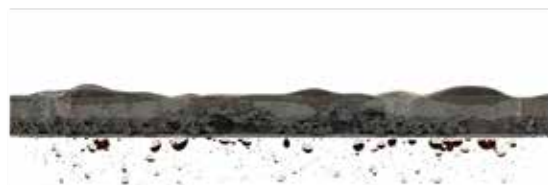
Conventional Flat Screen Solids Impede Fluid Flow
