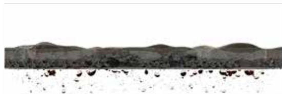
Conventional Flat Screen Solids Impede Fluid Flow
