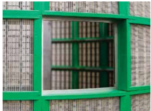
Replaceable cartridge removed from stainless cage
