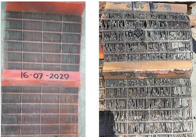
Figure 1 – Panel section before and after soaking for 3 days in slurry containing sulfuric acid and ammonia
