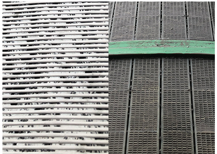
A side-by-side comparison of a wedge wire screen and G-Vault screen after operation.
