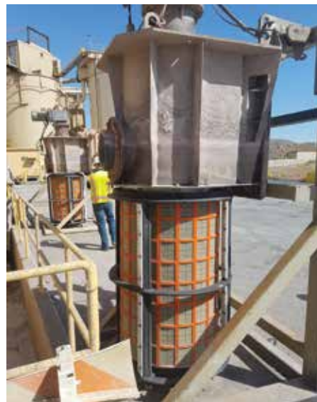
Figure 2 - G-Vault Interstage Screen pre-installation inspection
