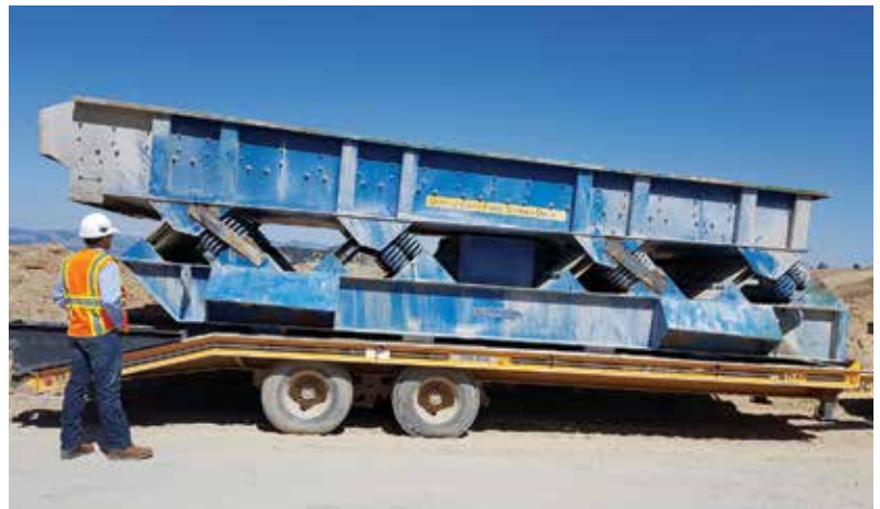
Removed original 8 ft x 20 ft vibrating screen
