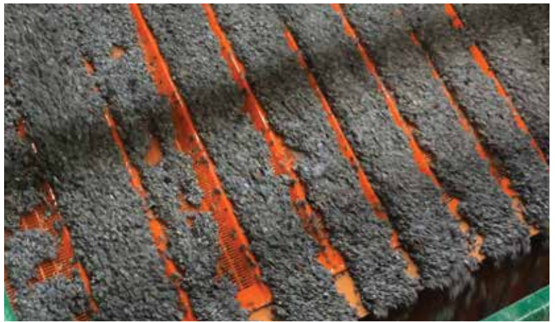
1.7 mm Derrick Polyweb urethane screen panel showing nonbinding surface.
