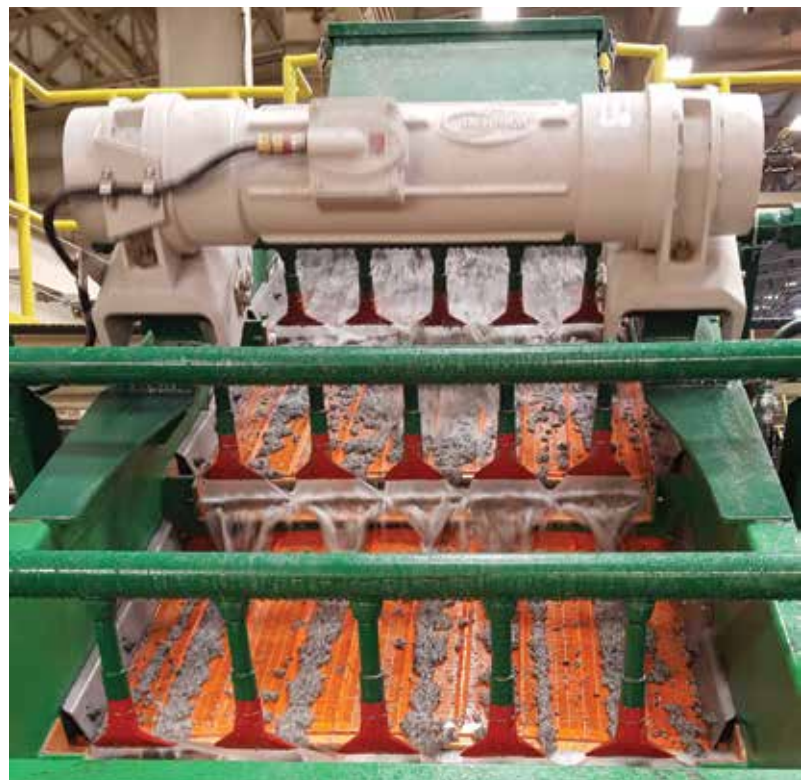
Downhill 4 ft x 10 ft Derrick Repulp Screen with a Super G® Vibrating Motor mounted on a single motor linear motion (SMLM) motor mount.
