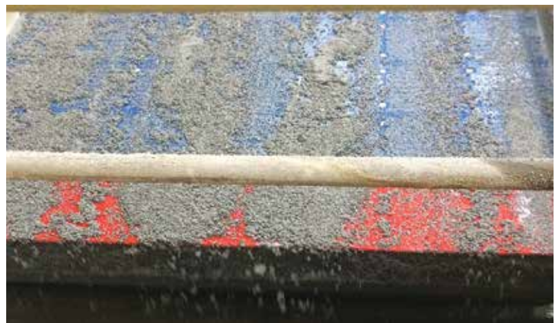
Original screen screen surface showing blinded panels
