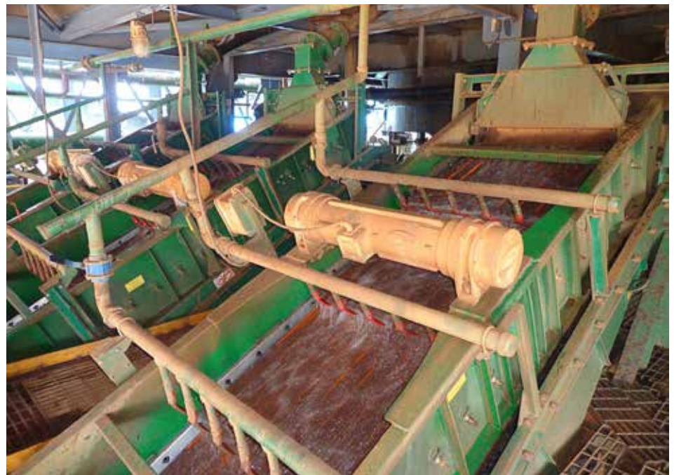
Derrick equipment is lighter and smaller than previously used conventional screening machines
