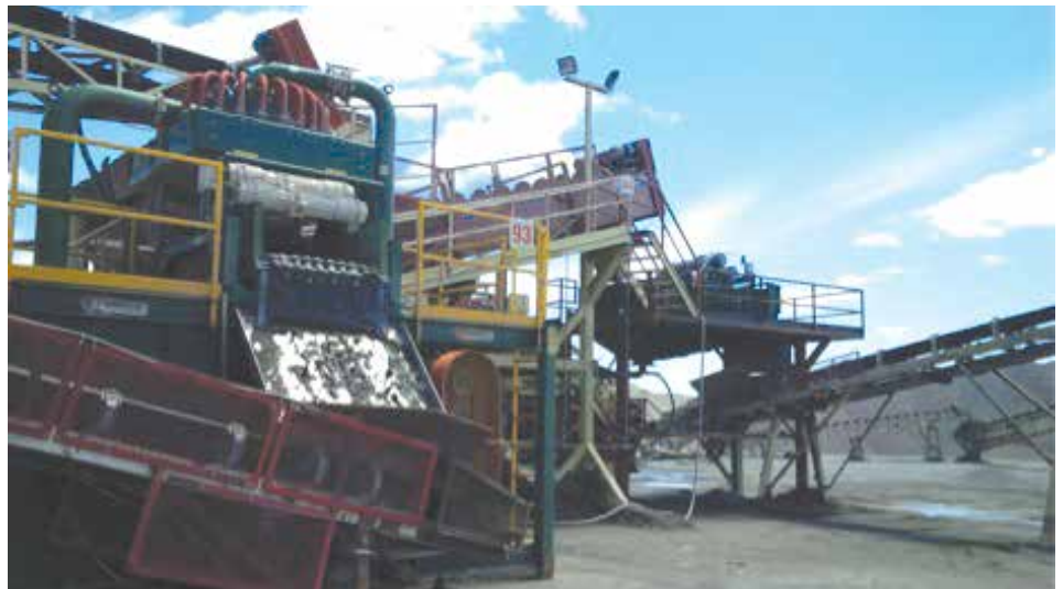
Derrick 4 x 8 HI-G ® Dewatering machine, coupled with Derrick 4" hydrocyclones
