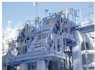
Derrick Corporation wet screening machines include a specialized unit for processing light, flaky, hard to convey solids. The Derrick Model 48-120W-4M High Shear Screener is a custom designed, open single-deck machine that can be operated in both non-hazardous and hazardous environments. This machine is typically used in wet sizing applications as fine as 325 mesh (45 microns) using Derrick Polyweb® urethane screens for kaolin clay, mica and fly ash.
