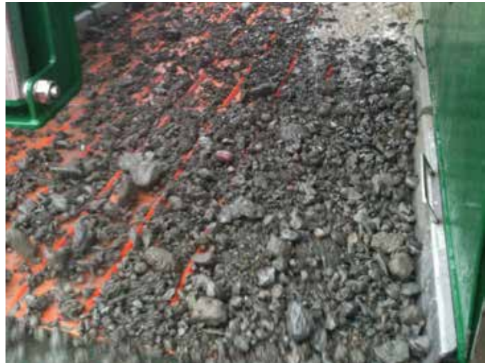
Derrick FLC 2000 operating with polyurethane screens
