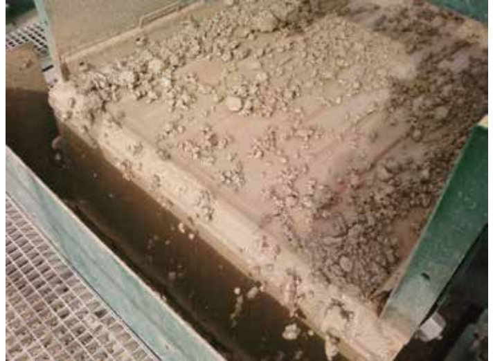
Derrick FLC 2000 handling primary separation
