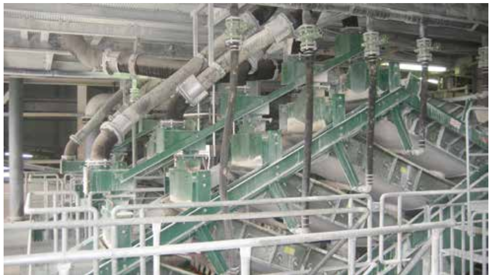
Derrick Stack Sizers have improved particle classification and increased cost savings
