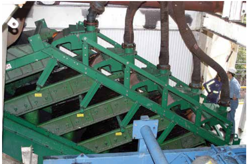
Figure 1. 5-deck Stack Sizer operating at Bevins Branch Preparation Plant
