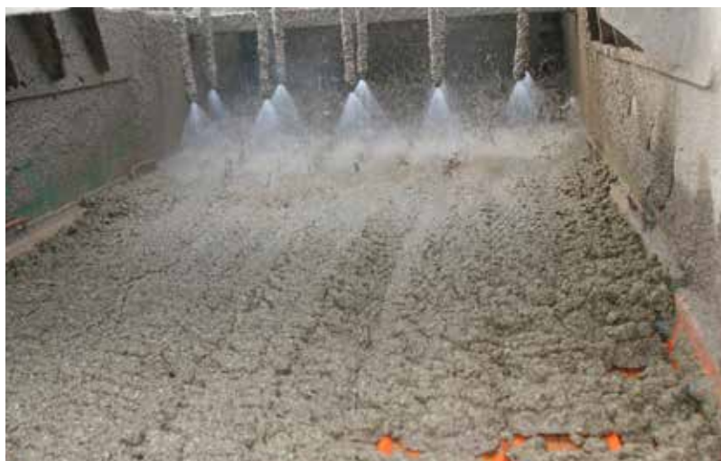
Linear motion machines fitted with high open area 25 mesh Polyweb urethane screen panels
