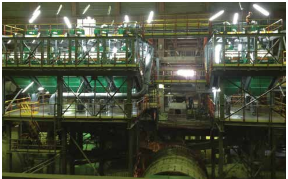
60 Stack Sizers at A.O. Apatit have dramatically increased plant performance by improving particle size separation
