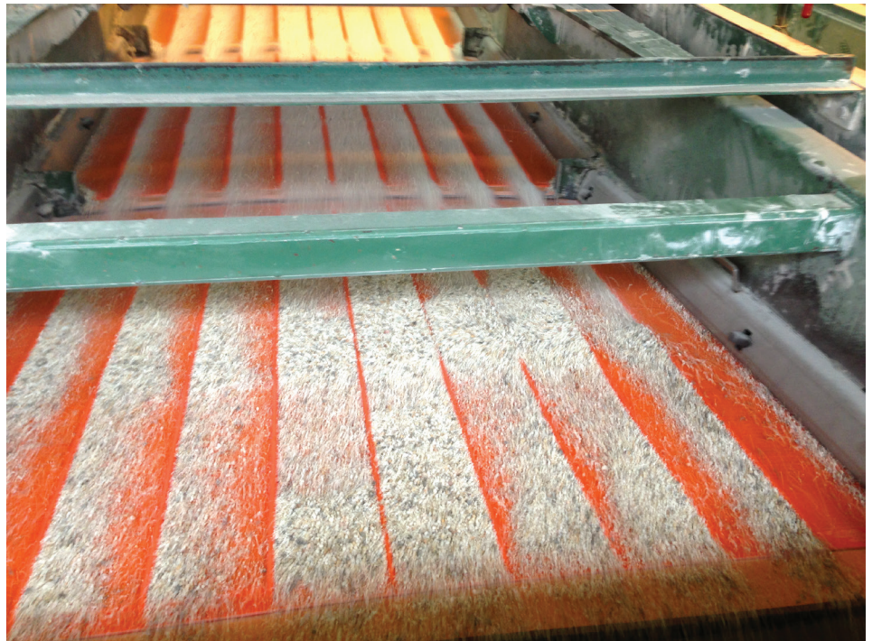
Polyweb DU panels classifying dry hydraulic fracturing sand. Polyweb DU panels are available in both standard rectangular openings and "sq" square openings.
